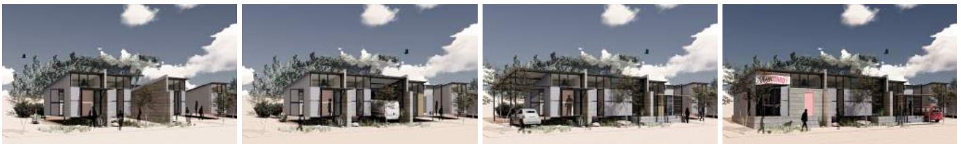
Development stages from left to right: Emergency response core unit with brick firewalls on narrow plots; incremental expansion, transformation, brick infill, livelihoods opportunities and street formation.
