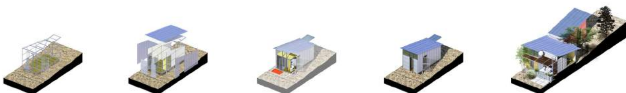
Design principles: [1] Modular steel frame; [2] Metal cladding, insulation and interior panelling; [3] Service core; [4] Core unit (emergency response); [5] Future potential for expansion.
